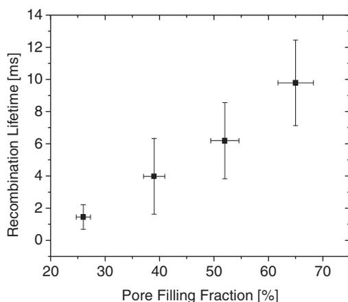
**Figure 5.** Recombination lifetime vs. PFF at short-circuit ( $V = 0$ ) for 2- $\mu$ m-thick devices, obtained through transient photovoltage measurements at 100 mW cm<sup>-2</sup> white light intensity.
