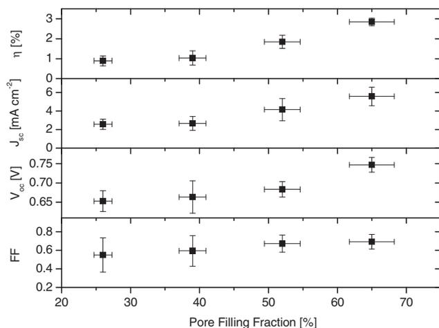
**Figure 1.** Current-voltage ( $I$ - $V$ ) characteristics for 2- $\mu$ m-thick devices at 1-sun illumination intensity (100 mW cm<sup>-2</sup>).
