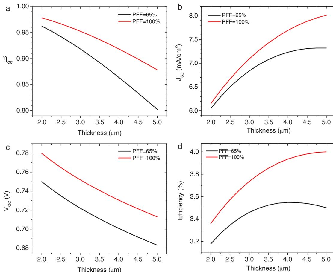
**Figure 8.** Modeled device parameters for Z907/spiro-OMeTAD system as a function of TiO<sub>2</sub> thickness for two different scenarios: PFF = 65% (black line), and PFF = 100% (red line). a) charge collection efficiency,  $\eta_{cc}$ ; b) short-circuit photocurrent,  $J_{sc}$ ; c) open-circuit voltage,  $V_{oc}$ ; d) power conversion efficiency.
