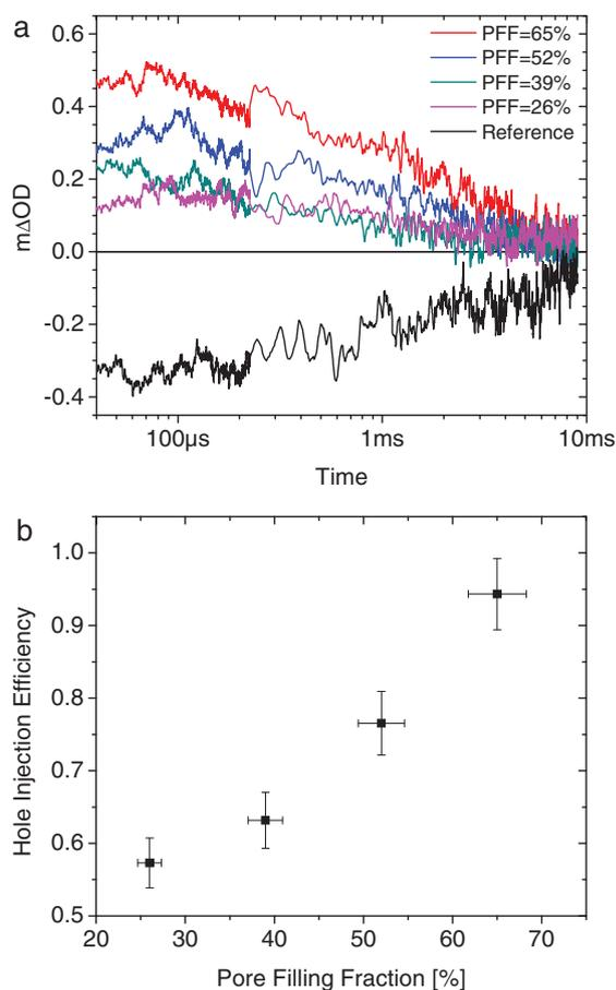
**Figure 3.** a) Change in optical density at 520 nm after excitation at 532 nm for 2- $\mu\text{m}$ -thick devices with different spiro-OMeTAD PFFs and one reference device with no spiro-OMeTAD; b) calculated hole injection efficiencies vs. PFF.
