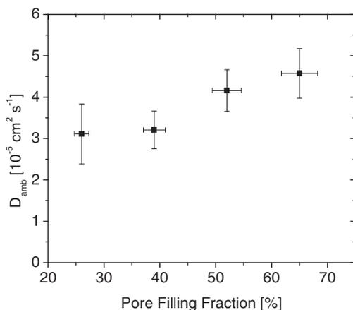
**Figure 6.** Ambipolar diffusion coefficient vs. PFF at short-circuit ( $V = 0$ ) for 2- $\mu\text{m}$ -thick devices, obtained through transient photovoltage and photocurrent measurements at  $100 \text{ mW cm}^{-2}$  white light intensity.
