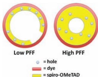
**Figure 4.** Schematic diagram showing the effect of the PFF on the spatial separation of holes from the dye-coated TiO<sub>2</sub> pore surface. Sub-monolayer coverage of dye molecules with HTM is shown in the case of low PFF. Real pores are not perfectly spherical as shown here.
