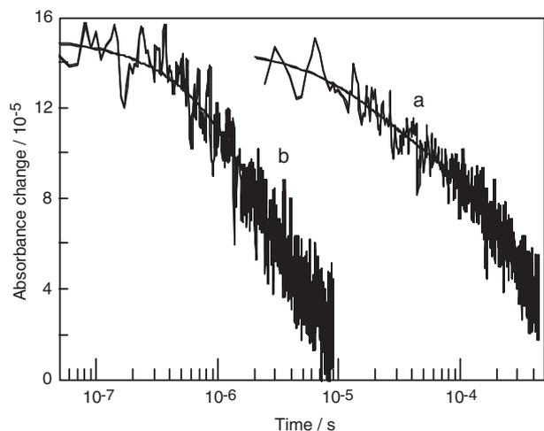
**Figure 5.** Transient absorbance decay kinetics of the oxidized state of Z-910 anchored on a nanocrystalline TiO<sub>2</sub> film a) in pure acetonitrile/valeronitrile (volume ratio: 3:1) solvent mixture and b) in the presence of the electrolyte used for device A. Absorbance changes were measured at a probe wavelength of 650 nm, employing 543 nm laser excitation (5 ns full width at half maximum pulse duration, 40 μJ cm<sup>-2</sup> pulse fluence).
