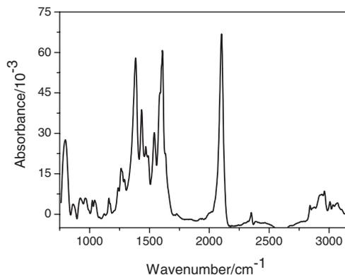
**Figure 4.** ATR-FTIR spectra for a 4  $\mu\text{m}$  mesoporous  $\text{TiO}_2$  film coated with Z-910 dye. A  $\text{TiO}_2$  reference film heated at  $500^\circ\text{C}$  to remove surface-adsorbed water has been subtracted for clarity of presentation.
