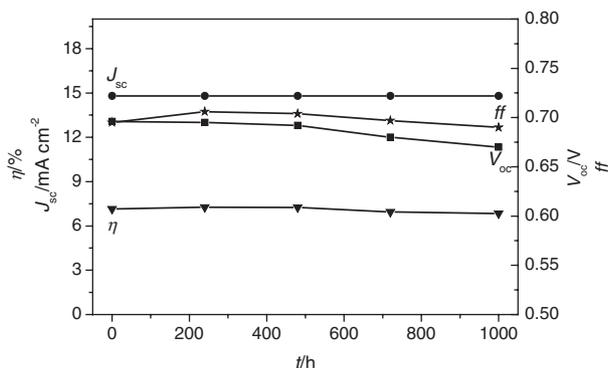
**Figure 7.** Detailed photovoltaic parameters of device B during successive one sun visible-light soaking at 55  $^{\circ}\text{C}$ .
