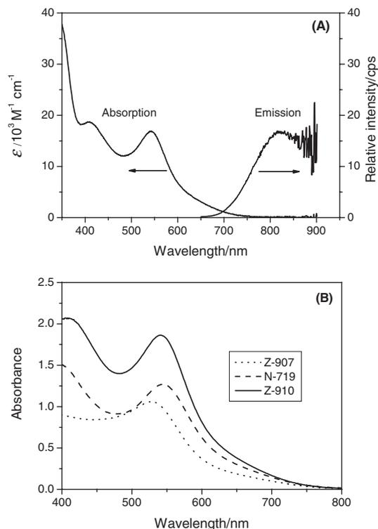
**Figure 3.** A) Electronic absorption and emission spectra of Z-910 dye in acetonitrile. B) Absorption spectra of Z-910, N-719, and Z-907 anchored on the 8  $\mu\text{m}$  thickness transparent nanocrystalline  $\text{TiO}_2$  film.
