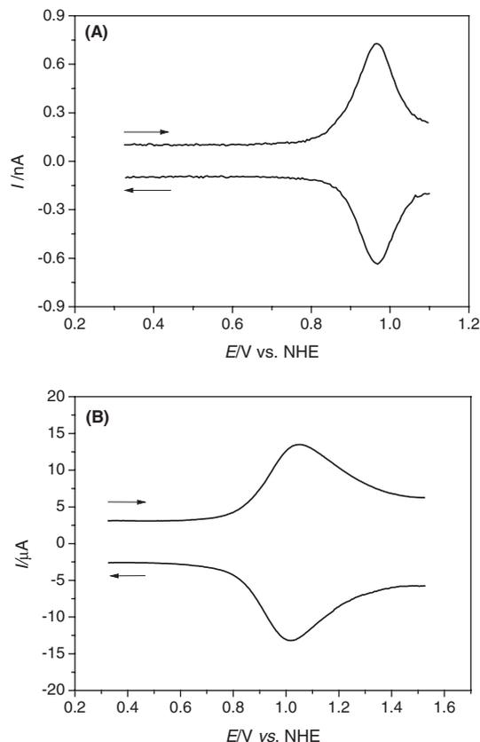
**Figure 2.** Square-wave voltammograms of A) a Pt ultramicroelectrode in DMF solution containing Z-910 and B) a nanocrystalline  $\text{TiO}_2$  electrode anchored with Z-910 in DMF. Supporting electrolyte: 0.1 M TBAPF<sub>6</sub>. Potential step increment: 10 mV; frequency: 25 Hz.
