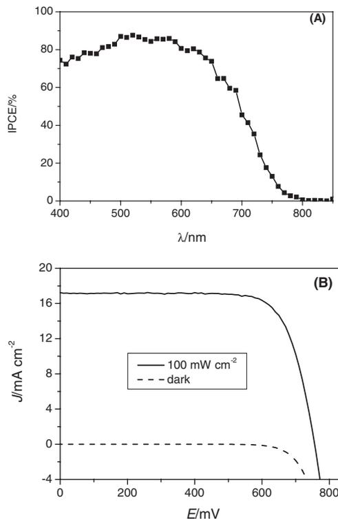
**Figure 6.** A) Photocurrent action spectrum of device A. B) Current density–voltage characteristics of device A under AM 1.5 sunlight (100 mW cm<sup>-2</sup>) illumination and in the dark. Cell active area: 0.158 cm<sup>2</sup>. Regions outside the active area are completely masked with black plastic to avoid the diffusive light.
