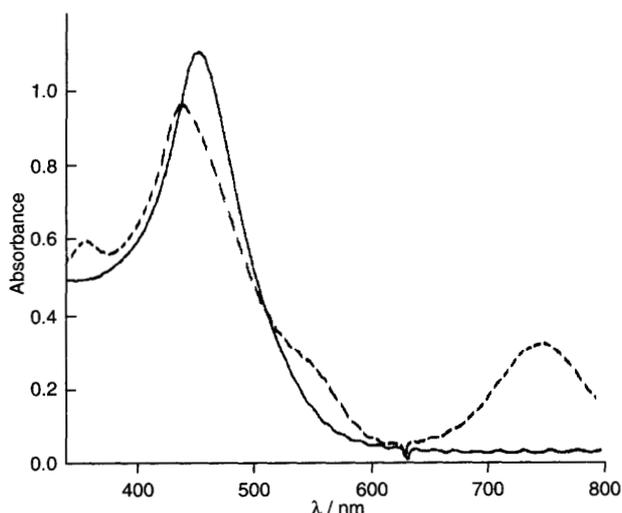
**Fig. 1** Photochromism of a nanocrystalline  $TiO_2$  film $\ddagger$  on  $SnO_2$  conducting glass, derivatized with a monolayer of complex **1**. The photoanode immersed in 1-ethyl-3-methyl bis[(trifluoromethyl)sulfonyl]amide was kept at +0.55 V. The initial spectrum (D-S, —) changed under illumination to the  $D^+-S$  spectrum (---). The original spectrum was regenerated by applying a potential of -0.3 V to the  $TiO_2$  electrode.
