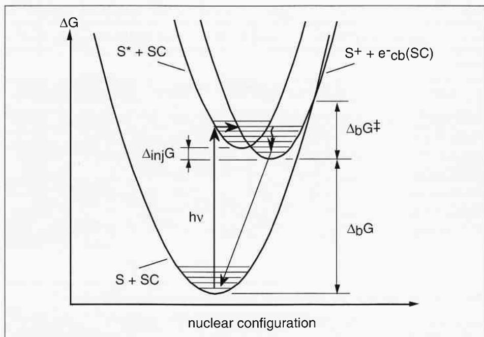
Fig. 1. Conceptual drawing showing free-energy surface crossing for interfacial charge-transfer processes depicted by Eqns. 2 and 3. While electron injection is kinetically nearly optimum ( $\Delta G^\ddagger \approx 0$ ), charge recombination falls deep into the inverted region. In the latter case, nuclear tunneling is likely to occur predominately, due to efficient contribution of the high-frequency vibrational modes and important Frank-Condon overlap.
