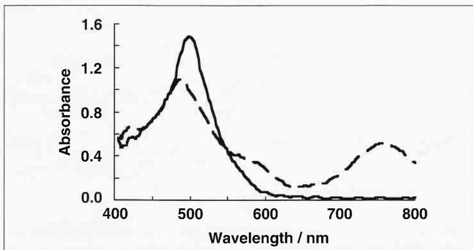
Fig. 2. Absorption spectra of the  $\text{TiO}_2$ -supported diad **1** in the dark (dotted line) and under white light illumination (solid line). Electrode was polarized in both cases at +0.55 V vs. NHE.
