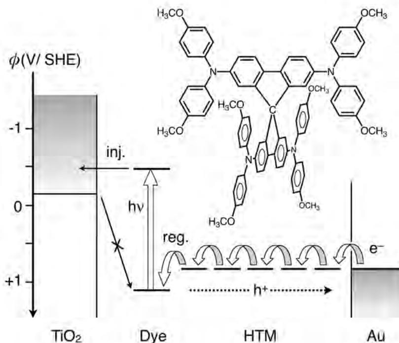
**Figure 11.25** Energetic scheme of electron transfer processes taking place in a dye-sensitized  $\text{TiO}_2$  | *spiro*-OMeTAD | Au heterojunction photovoltaic cell. Also shown is the molecular structure of the organic hole transporting material (HTM).
