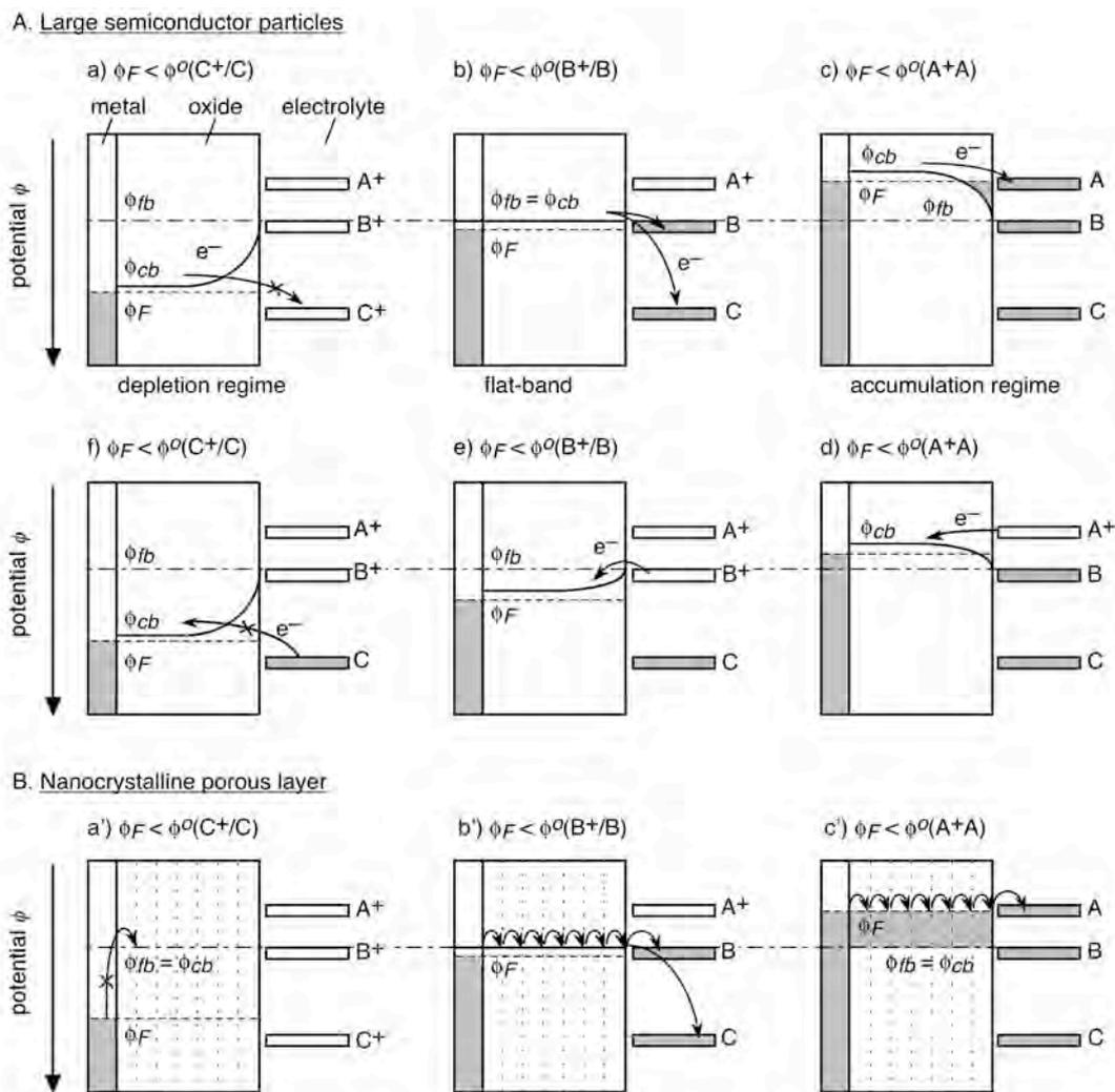
**Figure 11.4** Schematic representation of the interfacial electron transfer processes between the conduction band of a semiconductor and electroactive species on the surface, during the cyclic sweeping of the electrode potential (a)  $\rightarrow$  (b)  $\rightarrow$  (c)  $\rightarrow$  (d)  $\rightarrow$  (e)  $\rightarrow$  (f).
