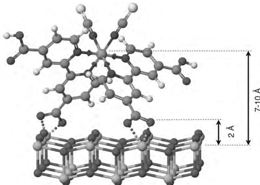
**Figure 11.15** Ball-and-stick molecular model of  $\text{Ru}^{\text{II}}(\text{dcbpy})_2(\text{NCS})_2$  dye adsorbed onto  $\text{TiO}_2$  anatase. While charge injection takes place from the  $\pi^*$  LUMO extending over the carboxylic anchors directly bond to surface  $\text{Ti}^{4+}$  ions, back ET returns the electron to the d-orbital (HOMO) localized on the  $\text{Ru}(\text{III})$  center, *ca* 7 Å apart from the surface.
