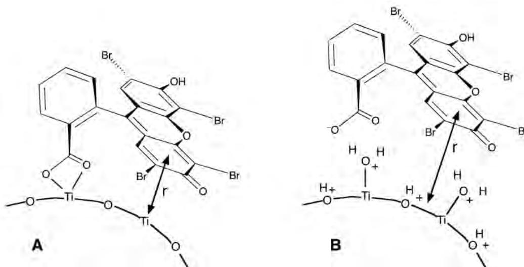
**Figure 11.3** Structure of the anionic form of eosin-Y dye adsorbed on the surface of dehydroxylated TiO<sub>2</sub> in a dry organic solvent (**A**), and on that of an hydroxylated oxide surface in acidic water (**B**). Tridimensional structure of the dye was obtained from a MOPAC semiempirical quantum mechanical calculation.
