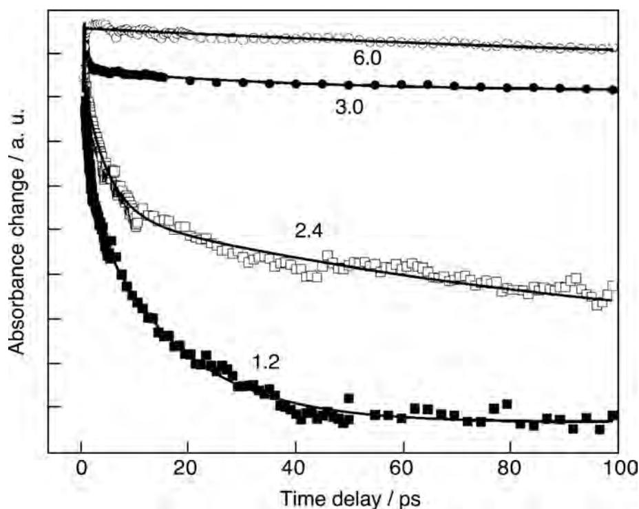
**Figure 11.14** Transient absorption decay of the photoexcited state of  $\text{Ru}^{\text{II}}(4'\text{-PO}_3\text{-tpy})(\text{NCS})_3$  dye adsorbed onto  $\text{Al}_2\text{O}_3/\text{TiO}_2$  core-shell nanocrystalline films measured by pump ( $\lambda = 530 \text{ nm}$ ) - probe ( $\lambda = 560 \text{ nm}$ ) fs laser spectroscopy. Alumina layer thickness was 1.2 nm, 2.4 nm, 3.0 nm, and 6.0 nm [73].
