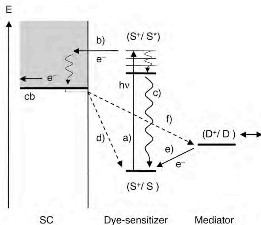
**Figure 11.1** Energetic scheme of electron transfer processes taking place after charge injection from a molecular electronic excited state S\* to the conduction band (cb) of a semiconductor (SC). Dashed arrows represent electron-hole recombination reactions that counter sustained charge separation.
