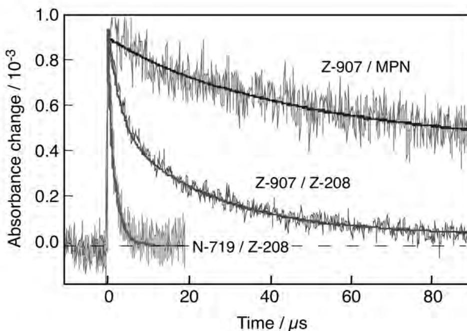
**Figure 11.23** Transient absorption decay kinetics of the oxidized state of N-719 and Z-907 dyes adsorbed on nanocrystalline  $\text{TiO}_2$  films in pure MPN solvent and in a non-volatile, lithium-free electrolyte, coded Z-908, containing  $[\text{I}^-] = 0.7 \text{ M}$  in MPN. Half reaction times measured for the systems Z-907/ MPN, Z-907/ Z-908, and N-719/ Z-208 are  $t_{1/2} = 180 \mu\text{s}$ ,  $15 \mu\text{s}$ , and  $200 \text{ ns}$ , respectively.
