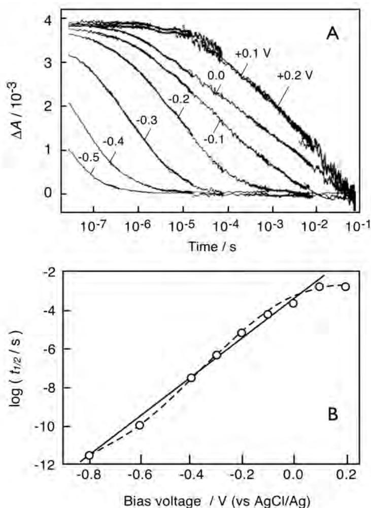
**Figure 11.20** (A) Transient absorption decay of the oxidized state of N-719 dye-sensitizer adsorbed on a TiO<sub>2</sub> nanocrystalline electrode under potentiostatic control. Dependence of the charge recombination kinetics upon the applied potential is shown for potentials ranging from +0.2 V to -0.5 V vs AgCl/Ag. (B) Dependence of the
