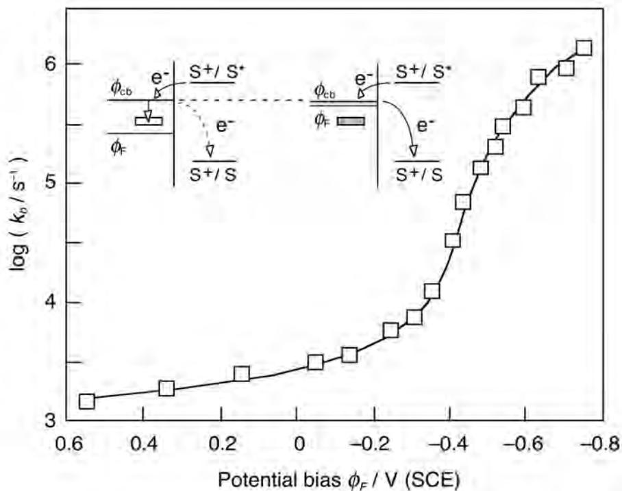
**Figure 11.6** Effect of the electrochemical potential bias applied to a nanocrystalline TiO<sub>2</sub> photoanode sensitized by Ru<sup>II</sup>(dcbpy)<sub>3</sub><sup>2+</sup> complex dye on the first order rate constant for the recombination of conduction band electrons with the oxidized sensitizer species Ru<sup>III</sup>(dcbpy)<sub>3</sub><sup>3+</sup>.
