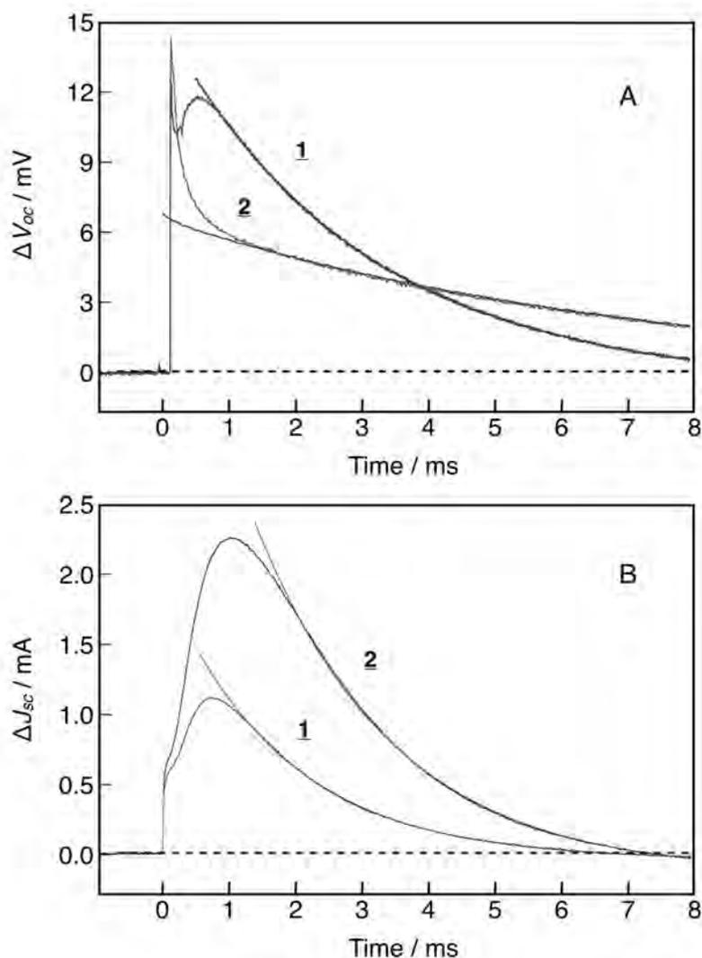
**Figure 11.26** Transient photovoltage (A) and photocurrent (B) of Z-907 dye-sensitized mesoporous  $\text{TiO}_2$  solar cells with electrolytes **1** and **2**. Lines superimposed on experimental signals are exponential fits of the decay processes. Data and conditions are that of ref. <sup>[120]</sup>.
