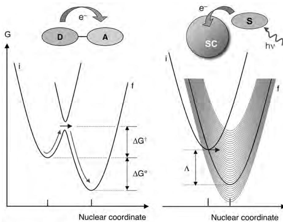
**Figure 11.8** Energetic situation for a typical vibration-mediated electron transfer between a donor (D) and an acceptor (A) described by Marcus theory (left) and the situation prevailing in the case of a continuum of acceptor states found in the dye-sensitization of a semiconductor (right).
