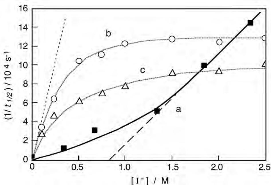
**Figure 11.24** Dependence of the pseudo first-order rate constant  $k_r' = 1/t_{1/2}$  of the regeneration of Z-907 (a, ■) and N-820 (b, ○) dyes adsorbed on nanocrystalline TiO<sub>2</sub> films upon I<sup>-</sup> concentration in MPN. Data points c (△) were obtained with N-820-sensitized TiO<sub>2</sub> and 0.5 M 1-methyl-benzimidazole base (NMB) added in the electrolyte. Data set a is from ref. <sup>[110]</sup>. Data points b and c are from ref. <sup>[109]</sup>.
