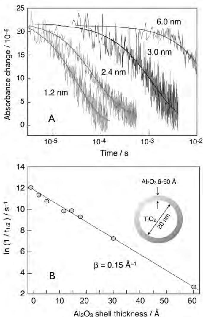
**Figure 11.19** (A) Transient absorption decay of the oxidized state of Ru<sup>II</sup>(4'-PO<sub>3</sub>-tpy)(NCS)<sub>3</sub> dye adsorbed onto Al<sub>2</sub>O<sub>3</sub>/TiO<sub>2</sub> core-shell nanocrystalline films. Alumina
