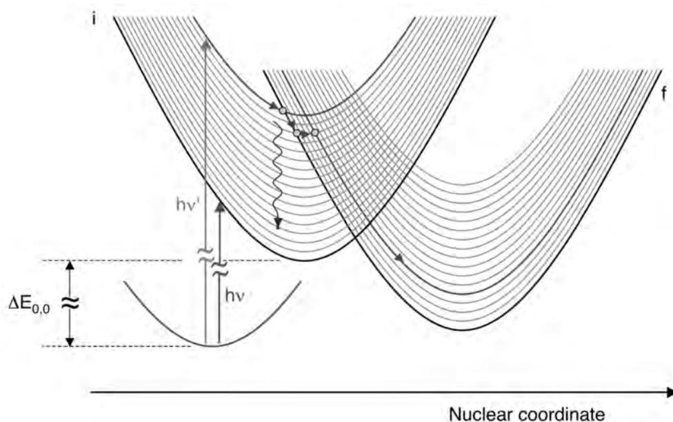
**Figure 11.9** Illustration of the competition between fast electron transfer from hot vibronic levels of a sensitizer and its vibrational relaxation. ET from the initial vibronic state prepared by absorption of radiation energy  $h\nu'$  has a smaller activation barrier than that excited by energy photons  $h\nu$  or obtained after vibrational relaxation to the lower level of the reactant state.
