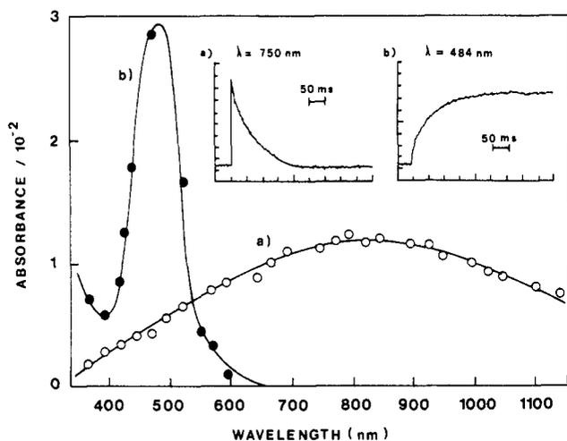
**Figure 2.** Transient spectra obtained from the laser photolysis of alkaline (pH 10) solutions of colloidal  $\text{TiO}_2$  (0.5 g/L) in the presence of  $5 \times 10^{-4}$  M **1** (concentration of PVA is 0.5 g/L):  $\circ$ , spectrum  $\sim 10 \mu\text{s}$  after the laser pulse;  $\bullet$ , spectrum 400 ms after the laser pulse. Insert shows temporal evolution of the absorbance at 750 and 484 nm.
