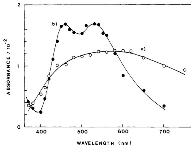
**Figure 4.** Transient spectra obtained from the laser photolysis of acid (pH 3) colloidal  $\text{TiO}_2$  solutions in the presence of  $2 \times 10^{-4}$  M **1** (concentration of  $\text{TiO}_2$  and PVA is 500 mg/L): (a) spectrum  $\sim 10 \mu\text{s}$  after the laser pulse; (b) spectrum 2 ms after the laser pulse.
