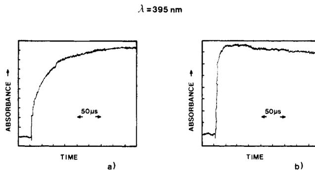
**Figure 6.** Oscillograms from the laser photolysis of colloidal  $\text{TiO}_2$  (0.5 g/L) in the presence of  $10^{-3}$  M viologenpropanesulfonate as electron acceptor, pH 3.5. No PVA protective agent was employed. Temporal evolution of the 395-nm absorption of reduced viologen is reported: (a) no  $[\text{Co}(\text{C}_5\text{H}_4\text{COO})_2]^-$ ; (b)  $[\text{Co}(\text{C}_5\text{H}_4\text{COO})_2]^- = 1 \times 10^{-5}$  M.
