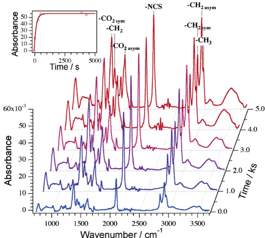
**Figure 2.** Dynamic ATR-FTIR spectra of staining of the TiO<sub>2</sub> nanocrystalline film with the Z-907Na sensitizer. Dye solution: 300  $\mu$ M Z-907Na in acetonitrile and *tert*-butyl alcohol (volume ratio 1:1). The temporal evolution of the thiocyanate absorbance (mOD) is shown in the upper left corner.
