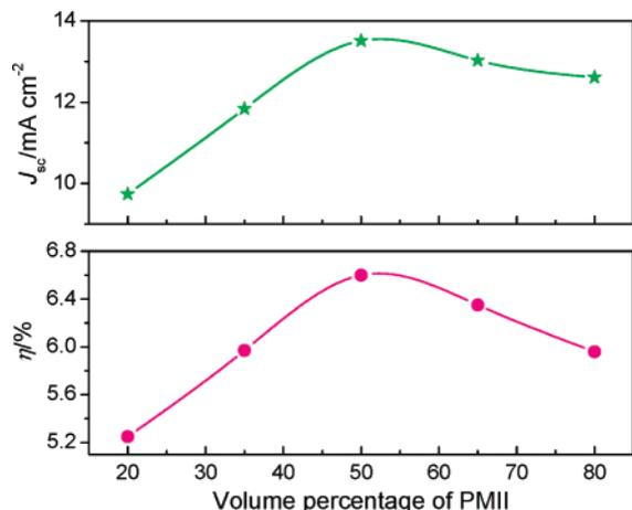
**Figure 6.** Dependence of photocurrent density and power conversion efficiency of devices under the AM 1.5 full sunlight ( $100 \text{ mW cm}^{-2}$ ) on the volume percentage of PMII. The iodine concentration is kept at  $0.2 \text{ M}$ .
