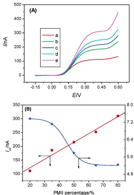
**Figure 5.** (A) Steady-state voltammograms of a Pt ultramicroelectrode in the binary mixtures of PMII and EMITCM. PMII volume percentage: (a) 20%; (b) 35%; (c) 50%; (d) 65%; (e) 80%. (B) Dependence of steady-state current and iodide diffusion coefficient on the volume percentage of PMII in the binary mixtures.
