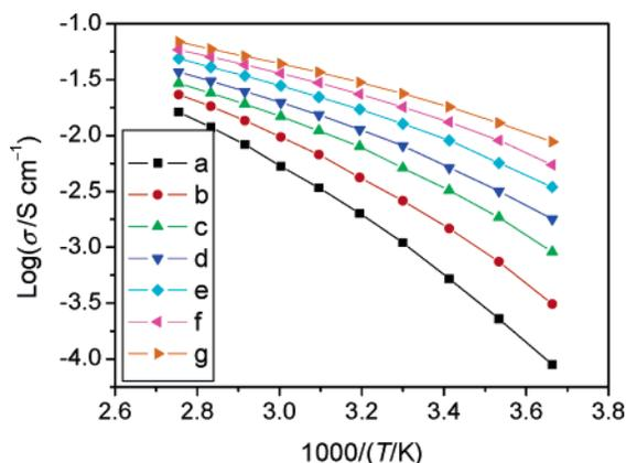
**Figure 4.** Conductivity–temperature plots in the Arrhenius coordinate for (a) PMII, (g) EMITCM, and binary mixtures (b–f) of PMII and EMITCM at different ratios. PMII volume percentage: (b) 80%; (c) 65%; (d) 50%; (e) 35%; (f) 20%.
