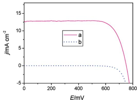
**Figure 8.** Current density–potential curves of devices with optimized binary ionic liquid electrolyte (a) under the AM 1.5 full sunlight and (b) in the dark. Cell area tested with mask:  $0.158 \text{ cm}^2$ .
