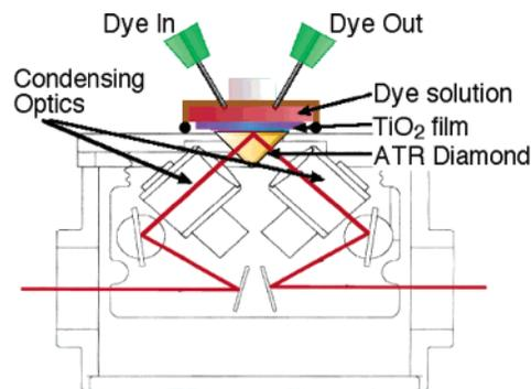
**Figure 1.** Schematic ATR-FTIR setup to monitor the dynamics of dye uptake onto nanocrystalline TiO<sub>2</sub> film.
