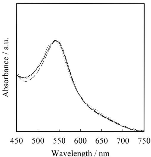
**Figure 2.** Absorption spectra of **1** in ethanol (···) and the same dye adsorbed onto the surface of a nanocrystalline TiO<sub>2</sub> (—) and ZrO<sub>2</sub> (---) films. Spectra were normalized to the absorbance maximum at 538 nm, after subtraction of the spectra obtained for undyed films, and were uncorrected for scatter.
