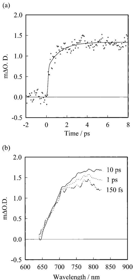
**Figure 7.** Subpicosecond transient absorption data obtained for the dye-coated  $\text{TiO}_2$  films. (a) Kinetics monitored at 750 nm. The solid line is a fit to the data, after deconvolution of the instrument response, corresponding to a  $1.2 \pm 0.2$  ps exponential growth, and a long-lived offset signal. (b) Transient spectra obtained at time delays of 150 fs, 1 ps, and 10 ps.
