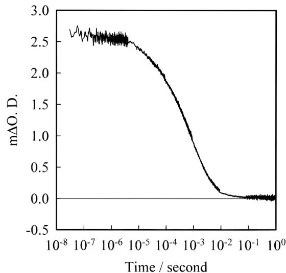
**Figure 6.** Kinetics of charge recombination in the dye-coated TiO<sub>2</sub> film, monitored by decay of the cation absorption band at 820 nm. The data are shown on a lin/log plot and exhibit multiphasic kinetics on the microsecond–millisecond time scales.
