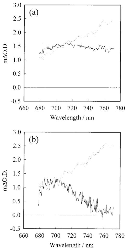
**Figure 4.** Transient absorption spectra obtained for  $\text{RuL}_2(\text{NCS})_2$ -sensitized  $\text{TiO}_2$  films (a) at time delays of 150 fs (—) and 60 ps (···) in the presence of 0.1 M  $\text{Li}^+$  (electrolyte A) and (b) at 150 fs (—) and 600 ps (···) in the absence of  $\text{Li}^+$  (electrolyte B). Other experimental conditions as for Figure 3.
