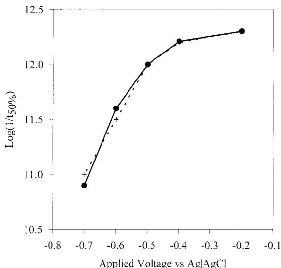
**Figure 6.** Comparison of the electrical potential dependence of the half time for electron injection,  $t_{50\%}$ , observed experimentally (+) with that calculated from nonadiabatic electron transfer theory as given by eq 1 (●). Details of the theoretical calculations are given in the Materials and Methods. The best fit to the experimental data, as shown (●) yielded fitting parameters of  $E_m = -0.75 \pm 0.05$  V vs Ag/AgCl and  $\lambda = 0.25 \pm 0.05$  eV.
