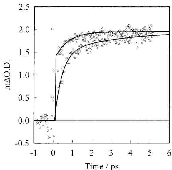
**Figure 3.** Transient absorption data for RuL<sub>2</sub>(NCS)<sub>2</sub>-sensitized TiO<sub>2</sub> films collected in the presence (circle) and the absence (triangle) of Li<sup>+</sup> in the electrolyte (electrolytes A and B, respectively) with a probe wavelength of 760 nm. The experimental conditions were the same as those presented in Figure 2 at an applied bias of  $-0.2$  V versus Ag|AgCl. Results of the kinetic fitting are shown as solid lines.
