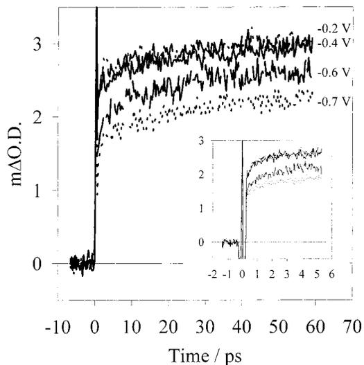
**Figure 5.** Transient absorption kinetics for  $\text{RuL}_2(\text{NCS})_2$ -sensitized  $\text{TiO}_2$  films collected at a probe wavelength of 760 nm, as a function of electrical potential applied to the  $\text{TiO}_2$  electrode. Data are shown for potentials between  $-0.2$  and  $-0.7$  V vs Ag/AgCl.
