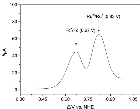
**Figure 2.** Square-wave voltammogram of the Z-907 dye anchored on the surface of interconnected TiO<sub>2</sub> nanocrystals. Potential step increment, 5 mV; amplitude, 20 mV; frequency, 10 Hz; scan rate, 50 mV s<sup>-1</sup>.
