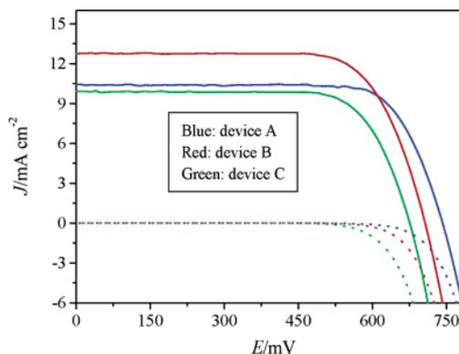
**Figure 4.** Current density–voltage characteristics of devices A–C at AM 1.5 (100 mW cm<sup>-2</sup>) illumination (solid curves) and in darkness (dotted curves). Cell active area is 0.152 cm<sup>2</sup>.
