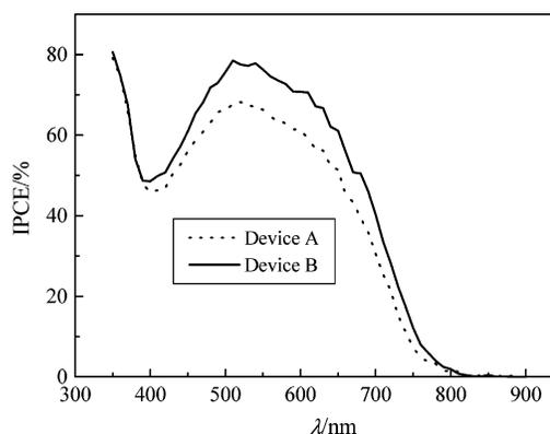
**Figure 3.** Photocurrent action spectra for devices A and B. Cell active area is 0.152 cm<sup>2</sup>.
