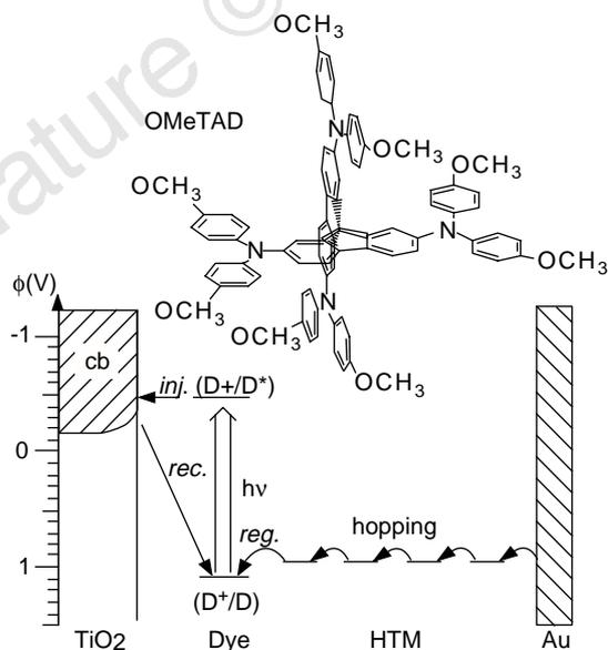
**Figure 1** Scheme for the electron-transfer processes (inj., injection; reg., regeneration; rec., recapture; hopping) occurring in the dye-sensitized heterojunction. Also shown are the approximate redox potentials and band energies of the different components.
